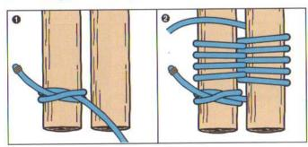
**Step 3**—Make eight to 10 loose wraps around the spars, then tighten the wraps with two frapping turns between the spars.
