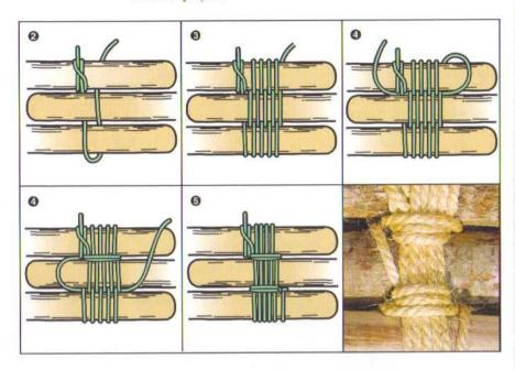
**Tripod Lashing.** A close relative of the shear lashing, the tripod lashing is the one to use for making a tripod or for joining together the first three poles of a tepee.
