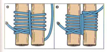
To make an A-frame trestle, place the spars next to each other and form a loose two-spar shear lashing about a foot from the top ends of the spars. Spread apart the other ends to form the A-frame, and tighten the lashing. See "A-Trestle," later in this section.
